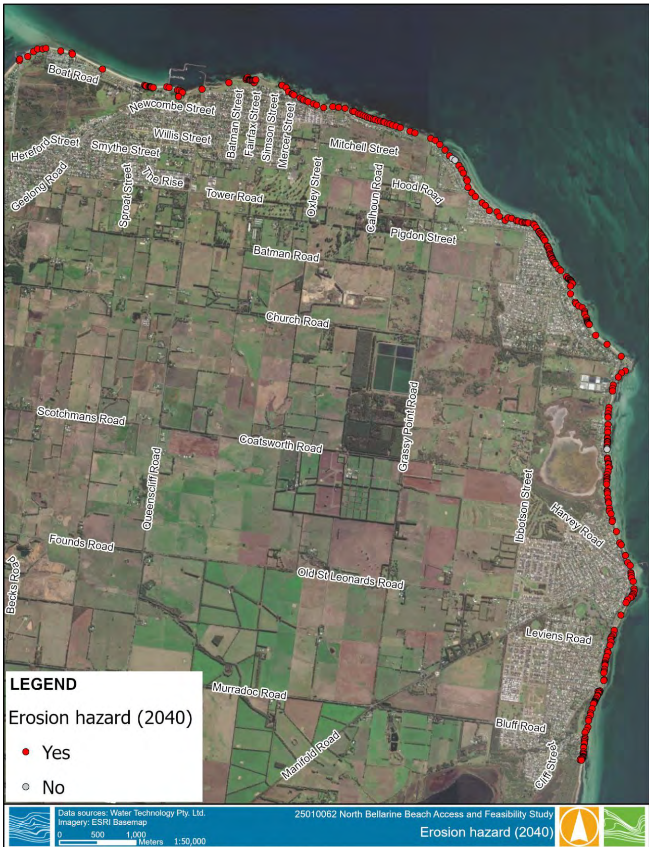
Figure 4-4 Beach Access vulnerable to erosion hazard in 2040 1% AEP storm
